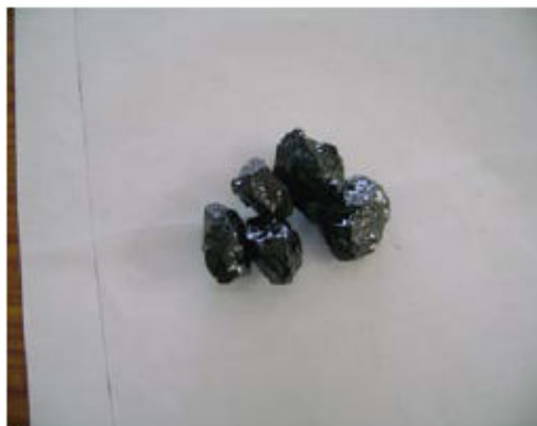
0.1% Zycosoil as anti stripping agent (98% adhesion) - 24 hr (97% adhesion) - 120 hr
