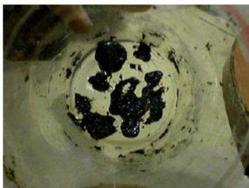
Asphalt stripped out after 48 hr ( Regular)
