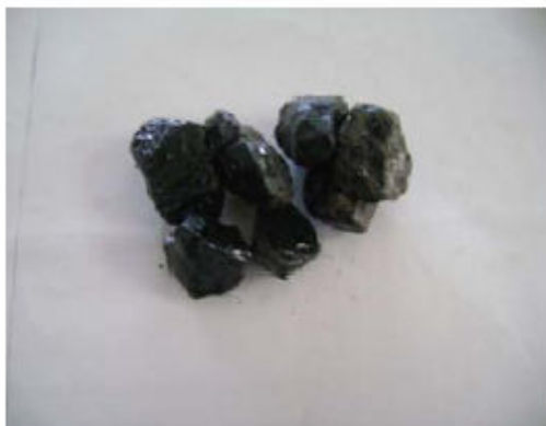
Normal aggregate (90% adhesion) – 24 hr (Failed completely)
